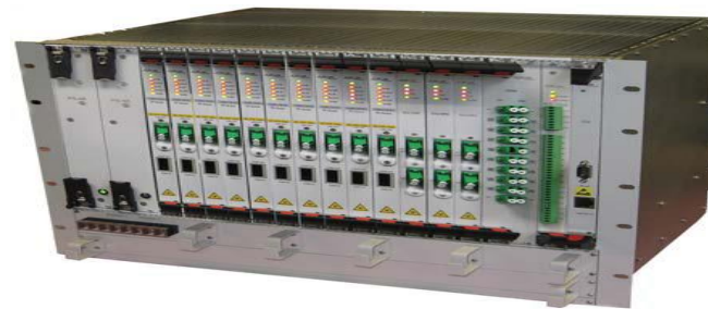
Ultra-Long-Haul DWDM System (Eliminates LAs & Repeaters from Spans >300 km)
